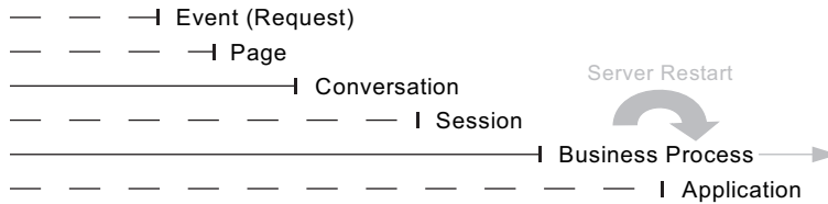
Figure 1.8 The lifetimes of the six scopes in a Seam application. The standard scopes are represented by dashed lines. The scopes that Seam contributes appear as solid lines. The business process scope is persisted to a database and can thus outlive the application scope across server restarts.
